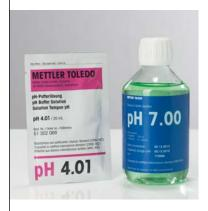
The internationally recognized pH scale is based on standard reference materials (SRM) selected by NIST (National Institute of Standards and Technology, USA). METTLER TOLEDO buffer solutions are traceable to these primary standards. The quality inspection certificate, that is available for every bottle and sachet, guarantees stated values and traceability.
