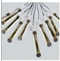
It is important to fill the reference electrode of every ISE with the recommended electrolyte solution. The correct electrolyte will minimize junction potentials and provide optimum temperature and time response. The electrolyte must be refilled or replaced regularly in order to achieve good electrode performance. For more information please refer to the electrode manual.
