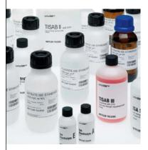
In all analytical procedures using an ISE, the correct amount of ISA (Ionic Strenght Adjustor) must be added to all samples and standards prior to measurement or calibration. This solution ensures that samples and standards have similar and constant ionic strength. Instructions for type and amount of ISA can be found in the manual of every ISE.
