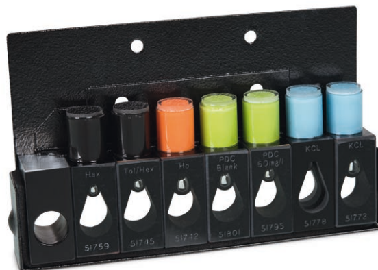
Inside CertiRef Sealed certified reference material (CRM) cuvettes
