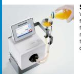
**Smart design** With a vertical design and a sampling funnel, the Easy Bev refractometer simplifies workflows. The throughput is maximized while minimizing sedimentation on the prism when measuring samples such as juices.
