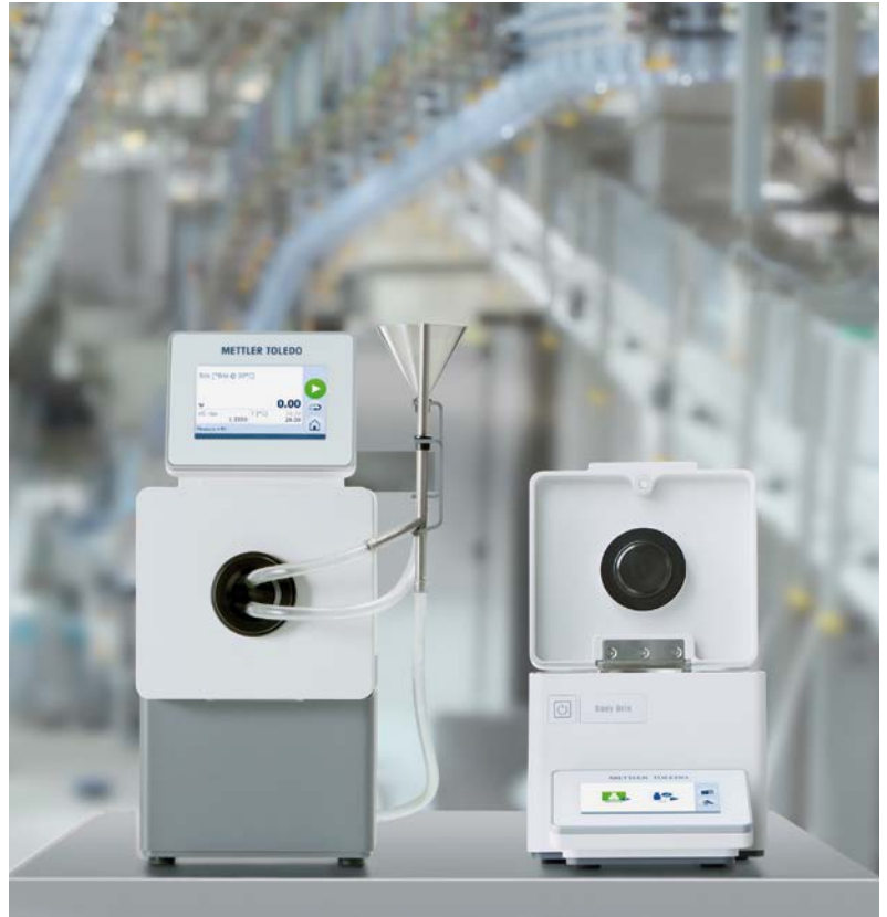
Figure 1. Sample preparation steps such as filtering and degassing can be avoided with the Easy Bev refractometer, while the Easy Brix and Easy R40 require low sample volumes. In each case, the instruments deliver results within seconds.
