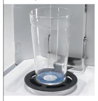
Remove transcription and ordering errors as well as improve efficiency with the new SmartSample RFID technology workflow. Identify and weigh your titration samples at an Excellence Analytical Balance with the SmartSample kit. Enter the sample identification (ID) at the balance to make sure the ID and weight are properly assigned to the physical sample.
