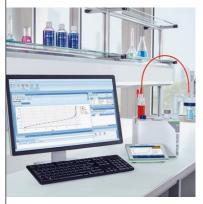
Each instrument connected to LabX has its own workbench correlating to that instrument. It offers all the components needed to run your daily tasks and the tools to monitor your sample series and results. Use the statistics view for quick and easy inspection of results to see if they are within established limits.
