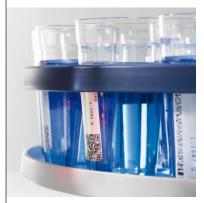
Fully automate the selection of the correct method and transcription of samples IDs with a barcode or SmartSample RFID tag. Thus, eliminate sample order errors by reading the sample information as you test it, as well as ensuring the right method is selected for each product. Use the automated 1D and 2D barcode reader with InMotion<sup>™</sup> Autosamplers.
