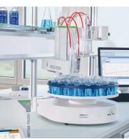
Use LabX to simplify sample changer operation with the transparent and easy-to-manage sample series tables. Track the state of your series from any LabX connected PC in your laboratory. Alter your series by adding or inserting urgent samples while operating.
