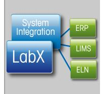
The relevance of system integration increases every year. With the Integration option of LabX 3<sup>rd</sup> party software such as ERPs, LIMS and ELN can easily be integrated. As an interface LabX offers API web service to exchange e.g. sample lists, start tasks and get the results back into your main system.
