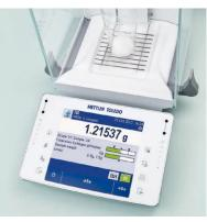
Excellence Balances connected to LabX have a dedicated entry point for titration tasks that require weighing. Simply pick the task and the balance will guide you through the samples. Start your titration and add more sample weights as you're testing for improved productivity.
