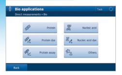
**Direct Bio measurements and methods** Bio UV/VIS applications can be started simply as direct measurements. Pre-verified METTLER TOLEDO Bio methods can be used for instant analyses or adapted with the intuitive editor to meet specific automation workflows. Both direct measurements and dedicated methods can be started by One Click<sup>™</sup> shortcuts.
