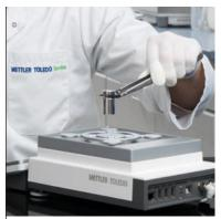
**3. Calibration and routine testing** Balance calibration is essential for accurate results. GWP® Verification service proves balance accuracy on-site and includes an optimal routine testing and calibration schedule, specification of the required test weights, and the ideal maintenance plan.
