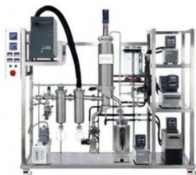
6" Stainless Turnkey Thin Film Distillation
